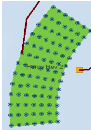
Figure 5-2 WTG layout at Horns Rev 2 designed to minimise the impact of changing wind direction on energy production [3]
